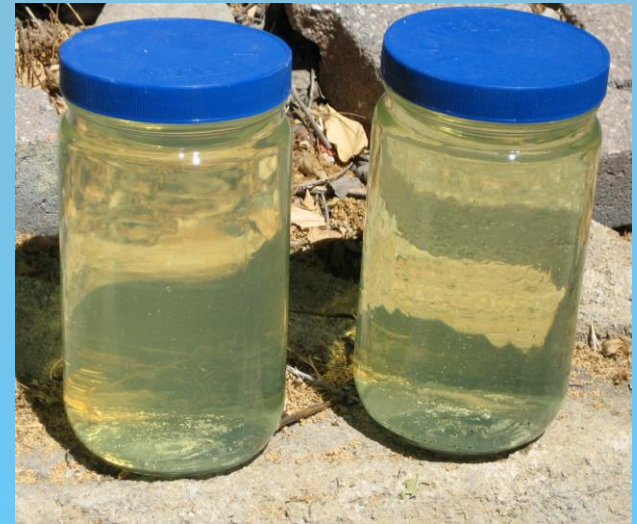
Colloidal sulfur remains in suspension in effluent
